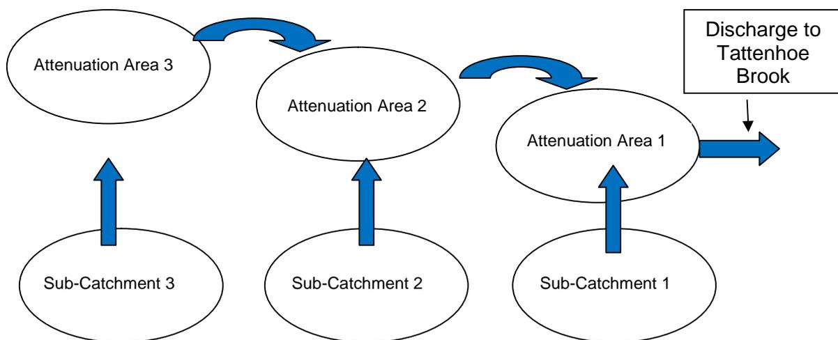
**Figure 4 – Cascading Attenuation System Draining Sub-Catchments 1 – 3**
